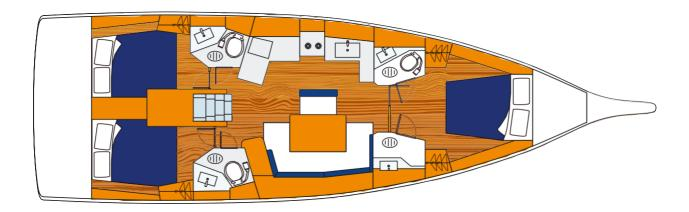
14.60m/47ft 9in Length Overall: Waterline Length: 13.65m/44ft 7in Beam: 4.50m/14ft 7in Draft: 1.75m/5ft 7in **Fuel Capacity:** 200L/52gal Water Capacity: 570L/150gal **Engines:** 80hp
